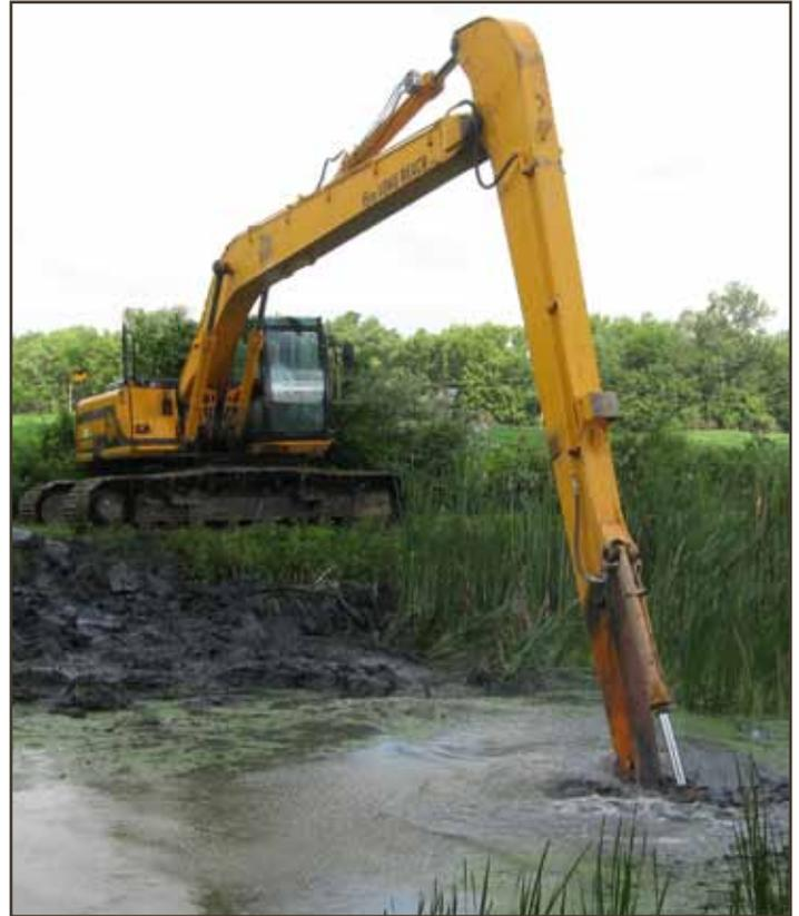
*Long reach excavator dredges the canal near 6-mile Spillway.*
